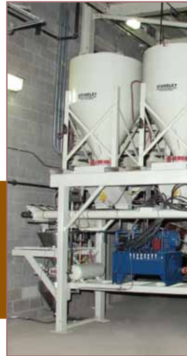
The dry-to-wet Standley Color Batch pigment metering system is an enclosed system that produces an unlimited range of colors.
